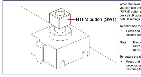
When the device is operational and linked to a network, you can use the Reset Test Function Management (RTFM) button (SW1 [see picture]) to announce the device's IP address or restore the device to the factory default settings.
