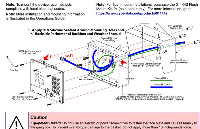
**Equipment Hazard**: Do not use an electric or power screwdriver to fasten the face plate and PCB assembly the gang box. To prevent over-torque damage to the gasket, do not apply more than 10 inch-pounds force. Over-torquing will cause the gasket to tear, risk moisture intrusion, and effectively void the manufacturer's warranty.
