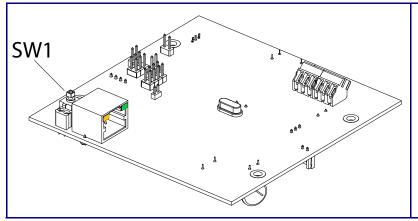
When the device is operational and linked to a network, you can use the Reset Test Function Management (RTFM) button (SW1) to announce the device's IP address or restore the device to the factory default settings.
