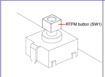
When the device is operational and linked to a network, you can use the Reset Test Function Management (RTFM) button (SW1 [see picture]) to announce the device's IP address or restore the device to the factory default settings.
