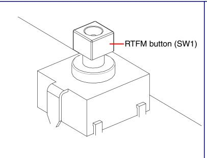
When the device is operational and linked to a network, you can use the Reset Test Function Management (RTFM) button (SW1 [see picture]) to announce the device's IP address or restore the device to the factory default settings.
