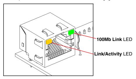
3.2. The green **100Mb Link** LED blinks off once during the boot up process when the device beings DHCP addressing and autoprovisioning attempts, and then comes on again and remains constant (solid green). The amber **Link/Activity** LED may be blinking depending on the network activity.
