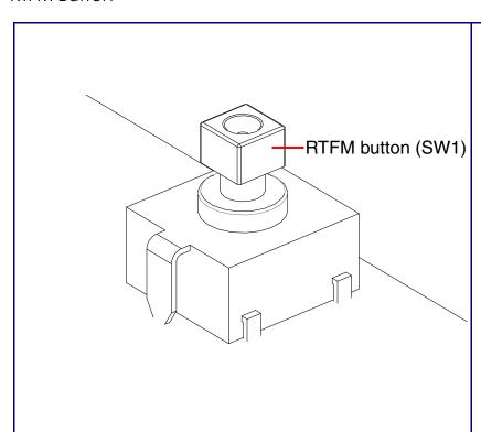
When the device is operational and linked to a network, you can use the Reset Test Function Management (RTFM) button (SW1 [see picture]) to announce the device's IP address or restore the device to the factory default settings.
