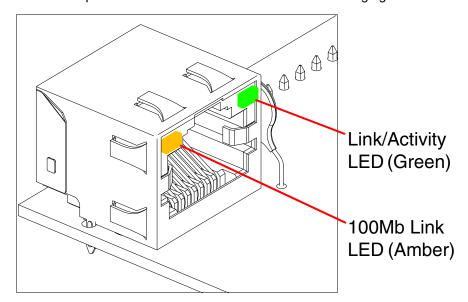
3.2. The green **100Mb Link** LED blinks off once during the boot up process when the device begins DHCP addressing and autoprovisioning attempts, and then comes on again and remains constant (solid green). The amber **Link/Activity** LED may be blinking depending on the network activity.
