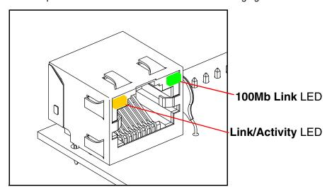
3.2. The green 100Mb Link LED blinks off once during the boot up process when the device beings DHCP addressing and autoprovisioning attempts, and then comes on again and remains constant (solid green). The yellow Link/Activity LED may be blinking depending on the network activity.
