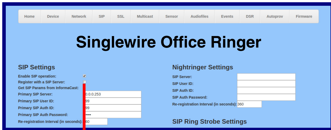
Figure 2-23. SIP Page Set to Point-to-Point Mode
