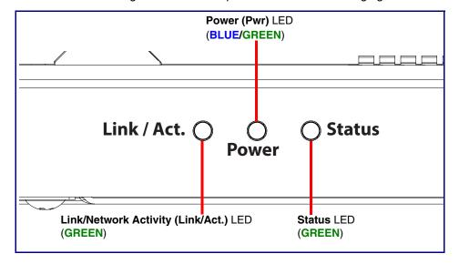
3.2. The Power (Pwr) LED is GREEN for 802.3af and is BLUE for 802.3at. The GREEN Status LED and the GREEN Power (Pwr) LED come on immediately. The Link/Network Activity LED blinks to indicate network traffic.
