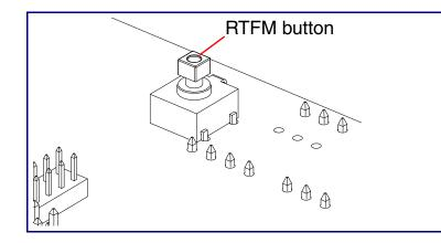
When the device is operational and linked to a network, you can use the Reset Test Function Management (RTFM) button (SW1) to restore the device to the factory default settings.
