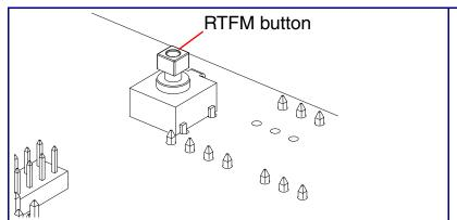
When the device is operational and linked to a network, you can use the Reset Test Function Management (RTFM) button (SW1) to restore the device to the factory default settings.
