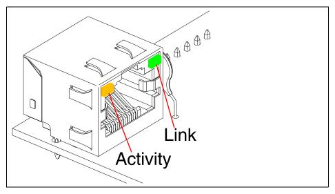
3.2. The **GREEN Link** LED blinks off once during the boot up process and then comes on again and remains constant (solid **GREEN**). The **YELLOW Activity** LED may be blinking depending on the network activity.
