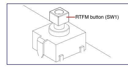
When the device is operational and linked to a network, you can use the Reset Test Function Management (RTFM) button (SW1) to restore the device to the factory default settings.
