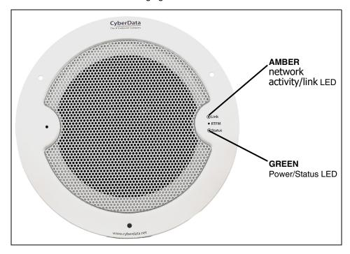
3.2. The **GREEN** Power/Status LED comes on immediately. The **AMBER** network activity/link LED will blink to indicate network traffic. After about 20 seconds, the **GREEN** Power/Status LED will blink twice to indicate that the board is fully booted.
