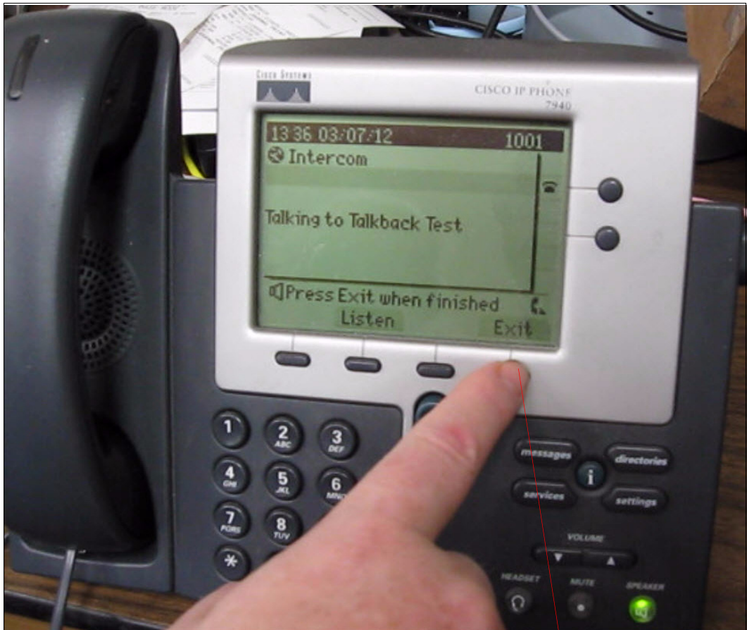
Figure 13. Press Exit to End to End the Call
