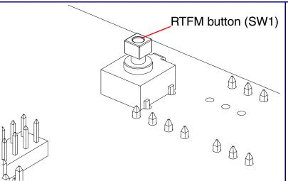
When the device is operational and linked to a network, you can use the Reset Test Function Management (RTFM) button (SW1 [see picture]) to announce the device's IP address or restore the device to the factory default settings.
