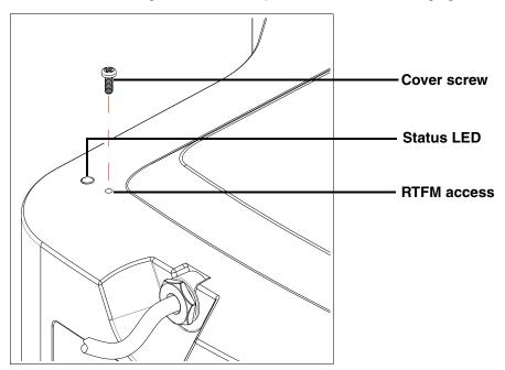
3.2. After about 20 seconds, the GREEN Status LED will blink fast to indicate that the device is acquiring an IP address and attempting to autoprovision. It will turn off thereafter until the device has finished booting. When the device has fully booted, the GREEN Status LED will turn on solid.
