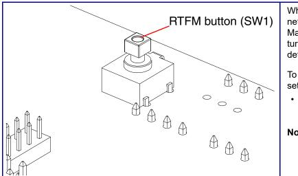
When the device is operational and linked to a network, you can use the Reset Test Function Management (RTFM) button (SW1 [see picture]) to restore the device to the factory default settings.
