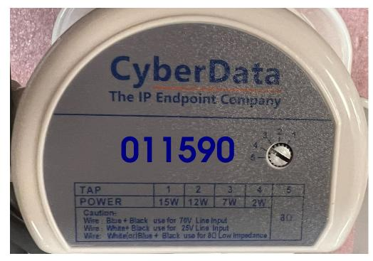
To connect constant voltage line inputs:
