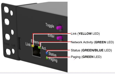
3.2. The GREEN/BLUE Status LED will blink during the boot process. The GREEN Paging LED will illuminate solid during initial network setup and then turns off. After the initialization process the GREEN/BLUE Status LED will blink twice a second.
